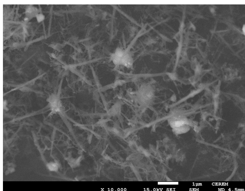
Figure 4: SEM image of Au-NRs synthesized by an aqueous mix of Olea europaea fruit extract and Acacia nilotica husk extract
