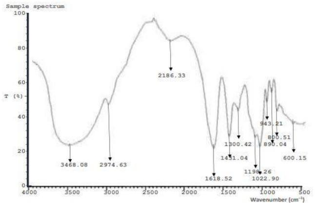
**Figure 7:** FT-IR spectrum of Emamectin Benzoate 5 – Control
