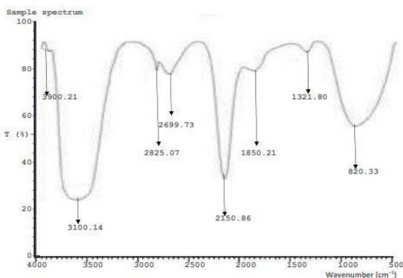
**Figure 10:** FT-IR spectrum of Emamectin Benzoate 5 degraded by *Bacillus subtilis*
