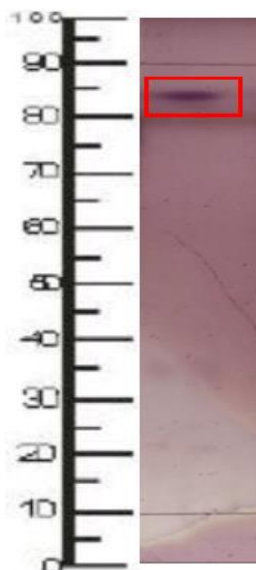
Figure 1: Compound identification using TLC. The TLC system used was as follows: mobile phase using n-hexane/ethyl acetate (8:2) and stationary phase using TLC plate GF60 254.
