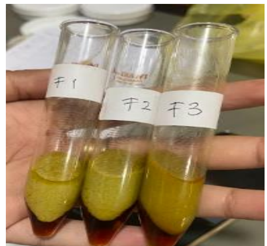
Figure 3: The centrifugation test results after 28 days.
