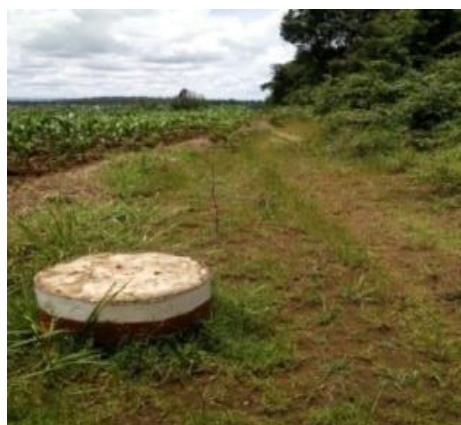
Plate 2: One of the beacons demarcating forest boundary in Nundu catchment forests (Photo by Manga)
