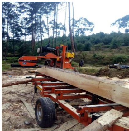
Plate 1: Sawing of logs into lumber using a Ding-dong machine (left) and a Wood-Mizer machine (right)
