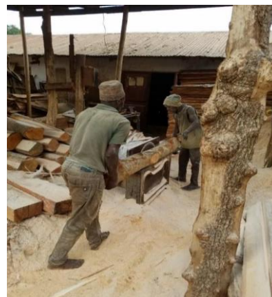
Plate 1: Sawing of logs into lumber using a Ding-dong machine (left) and a Wood-Mizer machine (right)
