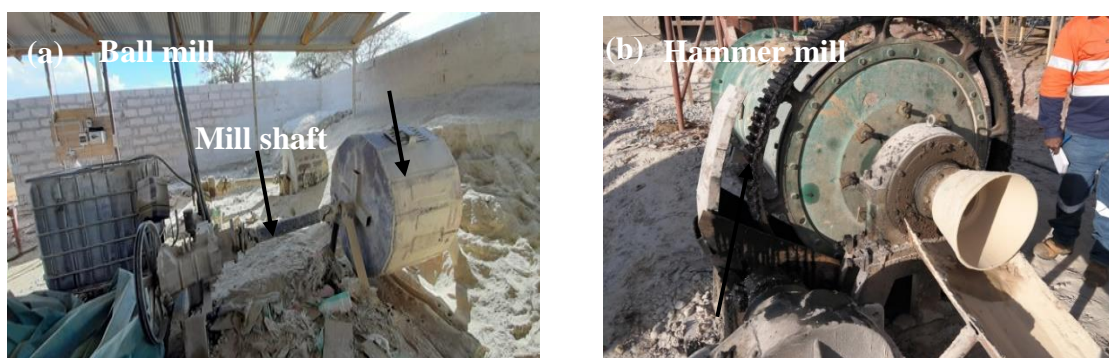
Figure 8: (a) Ball mills at Nholi mine (b) A hammer mill in Chunya mine.
