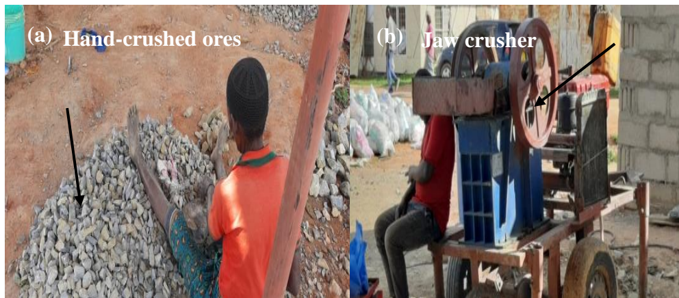
Figure 7: (a) Hand crushing (b) Jaw crushing operations at Nholi gold mine, Dodoma.
