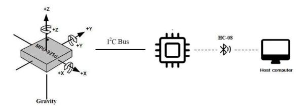
Figure 1: Schematic of hand-held somatosensory stick
