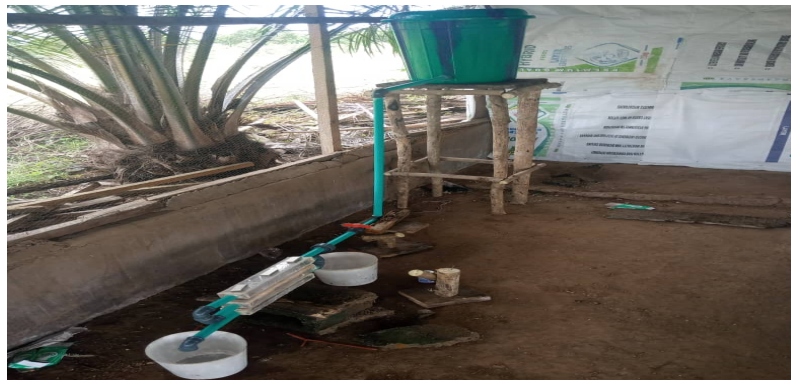
Figure 2 Pictorial view of the magnetic treatment unit for producing magnetized water
