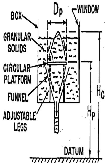
Figure 1: Schematic representation of the apparatus used for determination of angle of repose (Source : Mohsein, 1986)
