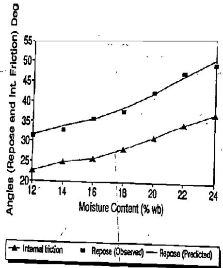
Figure 7: Angle of repose as a function of angle of internal friction and moisture content for data of wheat obtained from literature (Source: Sitkei, 1986)
