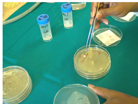
Figure III: Poly-Methylmethacrylate resins sample discs soaked in varying concentrations of AMS were placed in duplicate on spread plates of the different test organisms
