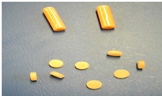
Figure 1: Prepared rods of Poly-Methylmethacrylate resins were sectioned into discs of 6.25 X 2mm.
