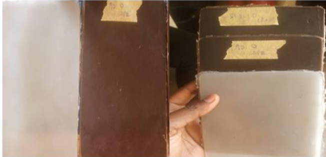
Figure 2. Press board samples of control (white) and LDPE/CP composites (brown)
