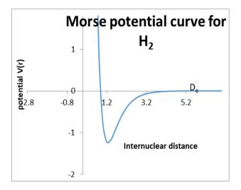
Figure 2: Morse potential curve for H2 diatomic molecule
