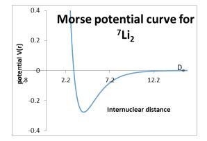
Figure 1: Morse potential curve for <sup>7</sup>Li<sub>2</sub> diatomic molecule.
