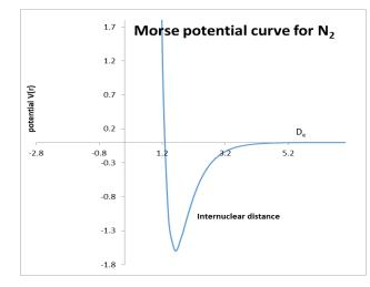
Figure 3: Morse potential curve for N2 diatomic molecule
