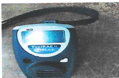
Plate 1: ToxiRAE Monitor for the measurement of Nitrogen dioxide
