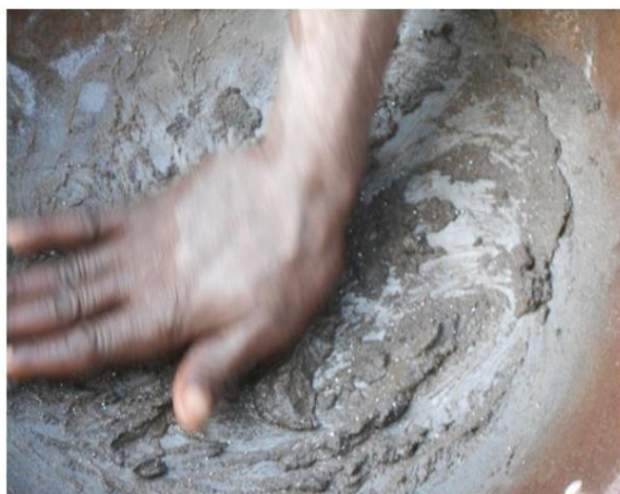
f. Mixing the residue with mercury metal
