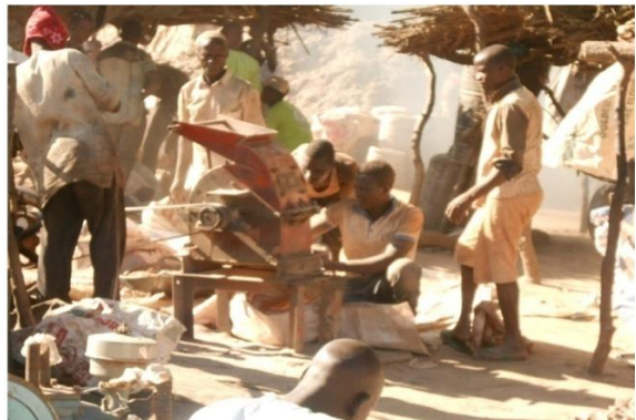
c. Grinding into powder the crushed rock materials
