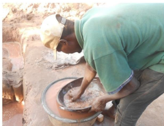
e. Further decantation process using head pan
