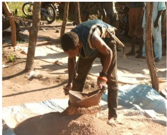
b. Sieving the crushed rock materials
