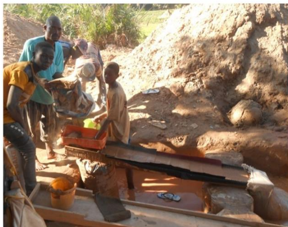
d. Separating Gold from sandy-dayey materials using decantation method
