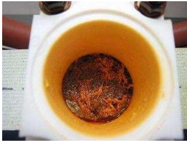
Figure 11. GFRP specimen after corrosion test with bromine.
