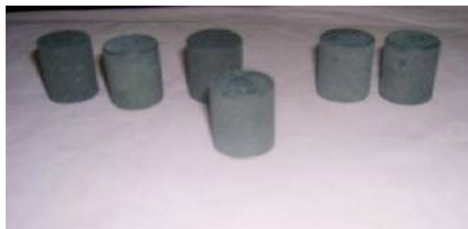
Figure 4: samples used for the measure of the hardness
