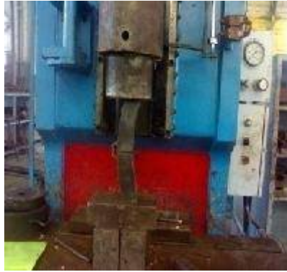
Figure 8: Device for the shear test on a hydraulic press
