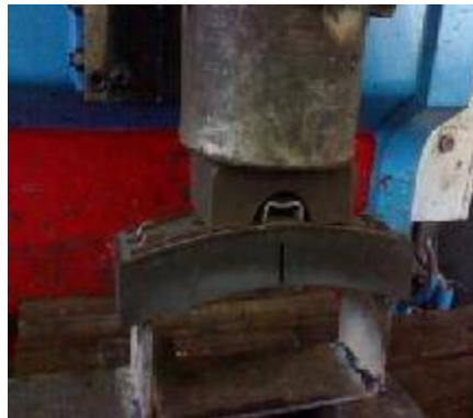
Figure 9: Application of the flexure test number 2
