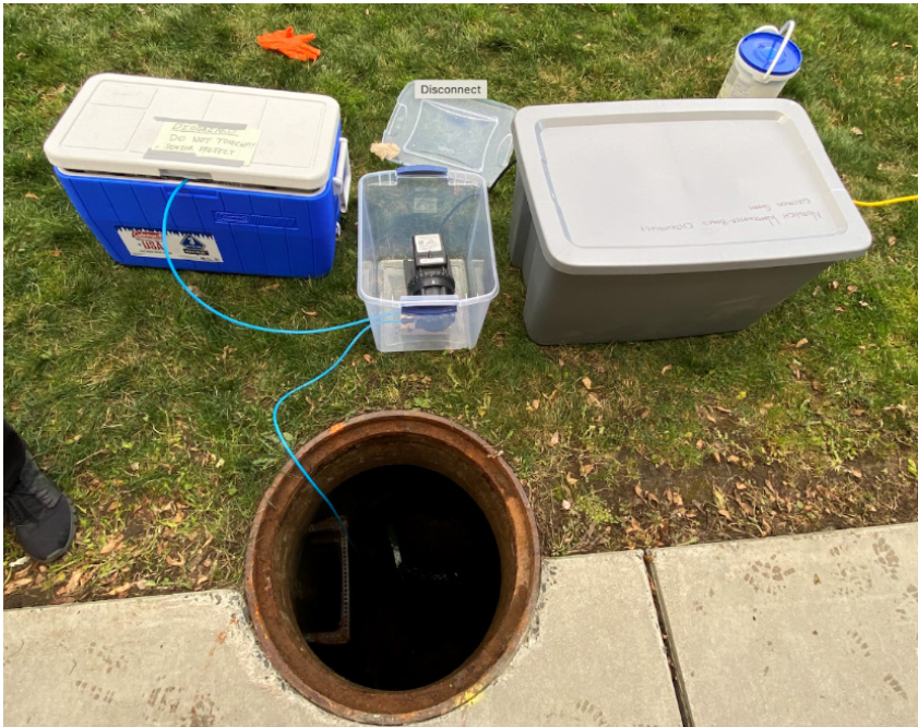
Figure 2. An automatic sampler designed and built by students to sample campus manholes for the SARS CoV-2 virus during the pandemic.
