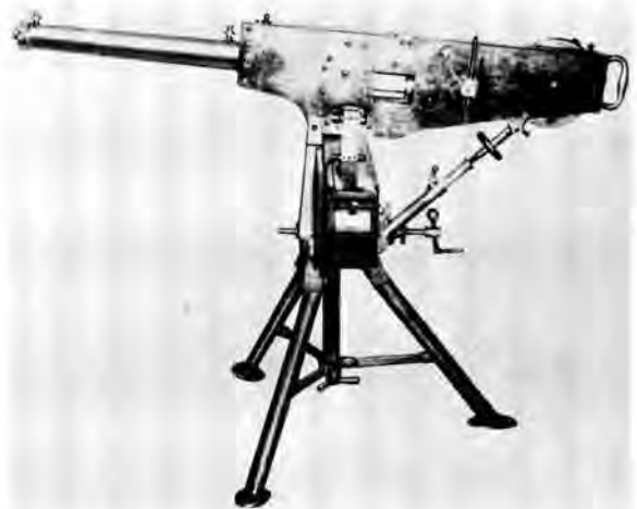
The 'first' Maxim model was designed in 1883 and was quite different to the model later marketed. It had a variable rate of fire from 1 to 600 rounds a minute. Without water it weighed 60 pounds.
