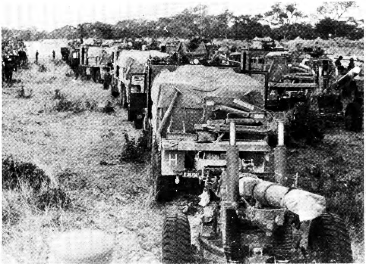
Alternative methods of towing the 140-mm gun. (above) – Marguris Deutz. (below) – Samil 100
