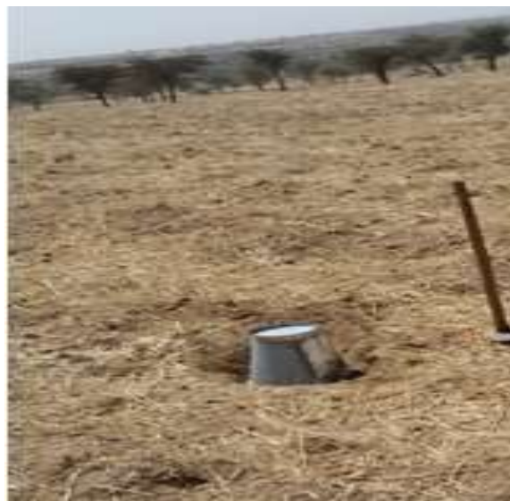
Figure 3. Single station measurement using TROMINO seismometer (TROMINO seismometer under the tan).
