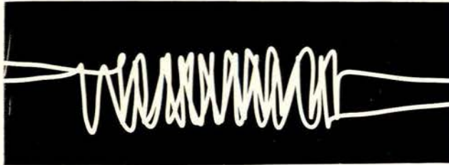
Fig. 16. Interlocking of 2 identical wire spirals shows a mixture of transverse and oblique elements due to summation in the 2-dimensional radiological image.
