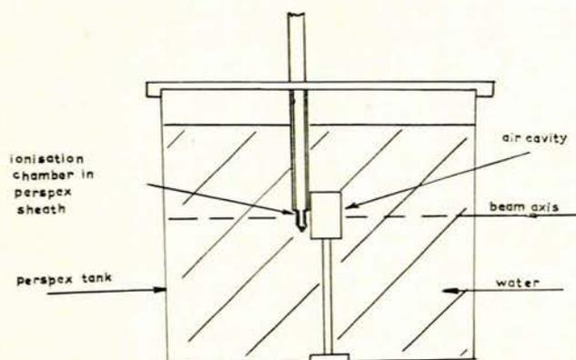
Fig. 2. Water phantom used in determining dosage variation.
