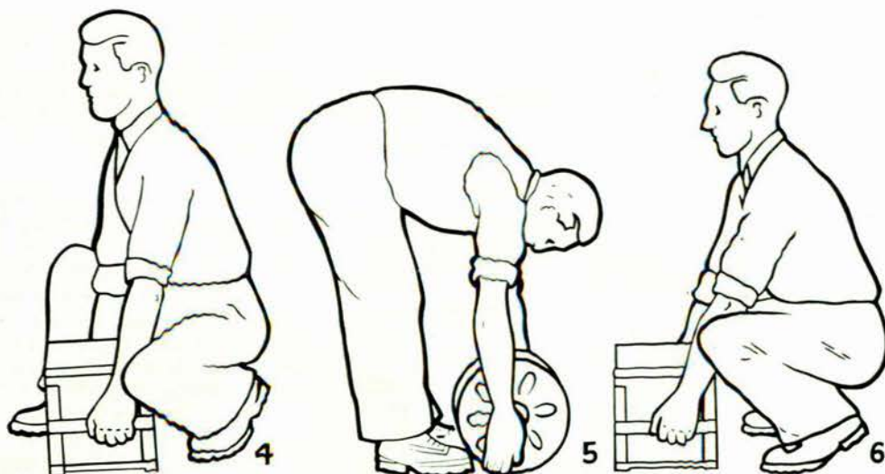
Fig. 4. The Kinetic posture when picking up a box: (1) chin tucked in, (2) back straight, (3) arms supported by thighs, (4) broad palmar grip, (5) knees relaxed, feet apart, and one placed in front of the other. Figs. 4, 5 and 6 are reproduced by permission of Imperial Chemical Industries.
