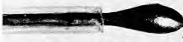
Fig. 1. View of end of stylus in polythene tubing (enlarged).
