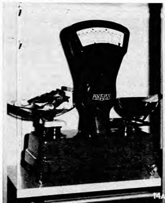
Fig. 14A. Scale for weighing used swabs to determine the amount of blood loss.
