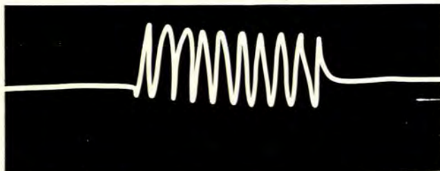
Fig. 15. Radiograph of wire spiral. For an uninterrupted transition from circular to longitudinal, a spiral arrangement is necessary.
