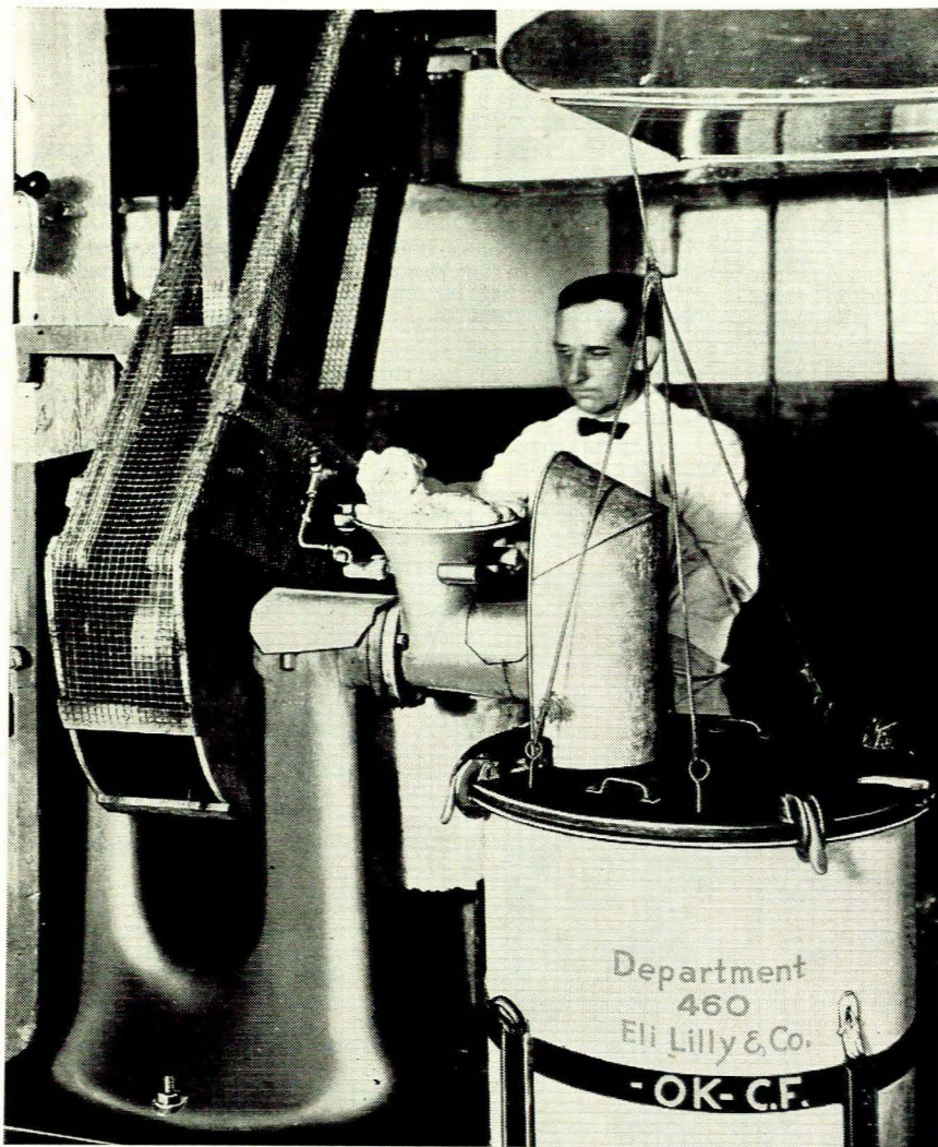
Fig. 2. Grinding of animal pancreas glands in 1923—the first step in insulin production.
