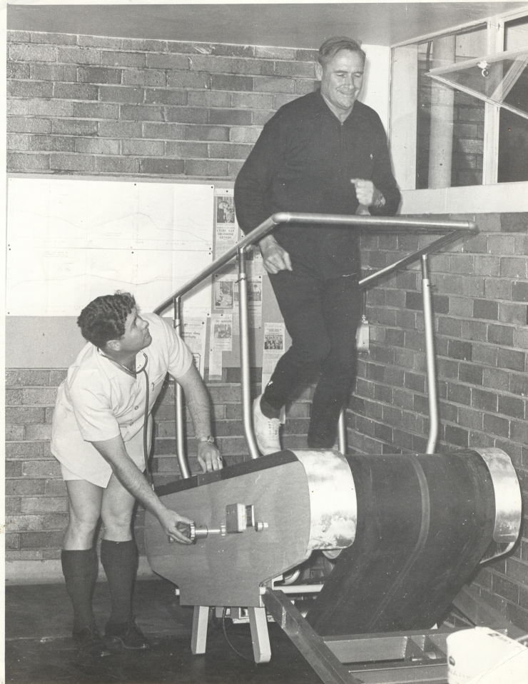
FIGURE 4. TREADMILL BUILT BY THE UNIVERSITY'S TECHNICAL DEPARTMENT. HYDRAULIC JACKS WERE USED FOR INCLINE AND DECLINE ADJUSTMENT
