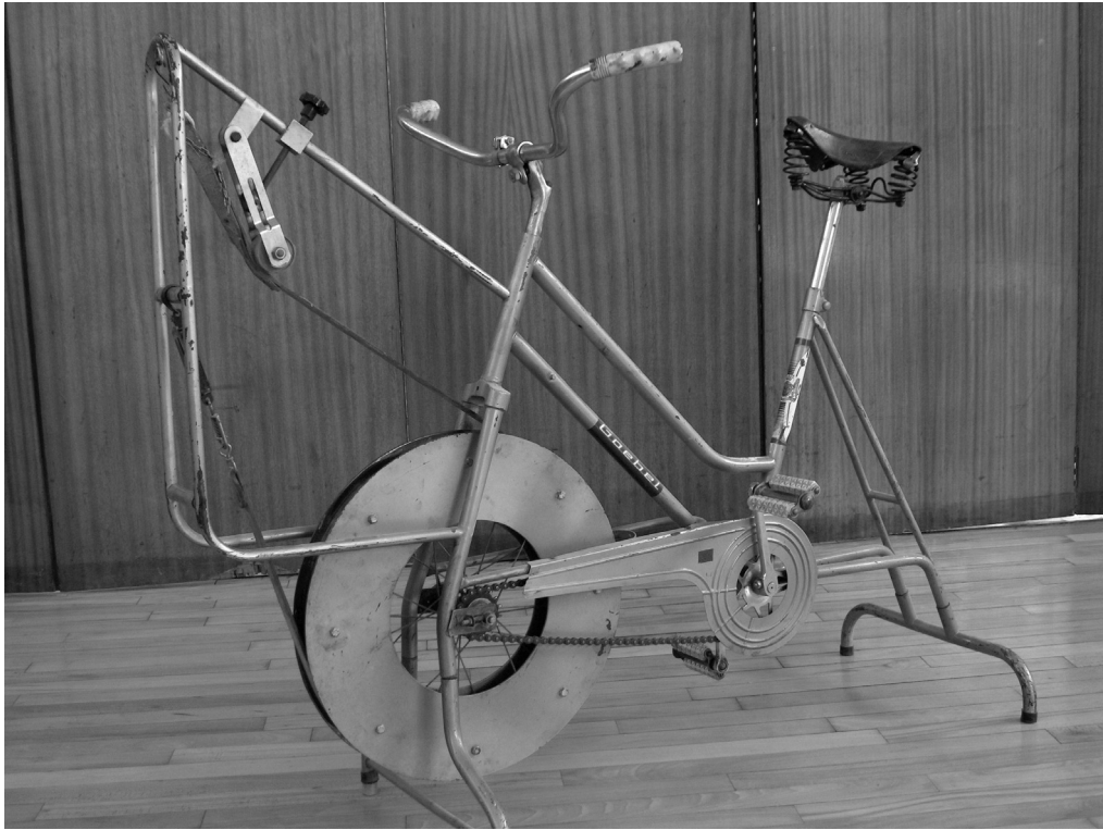
FIGURE 3. MODIFIED BICYCLE ERGOMETER TO MEASURE WORK CAPACITY. NOTE THE LEATHER BELT ON THE FLYWHEEL AND THE KITCHEN SPRING BALANCE WHICH MEASURED THE WORKLOAD
