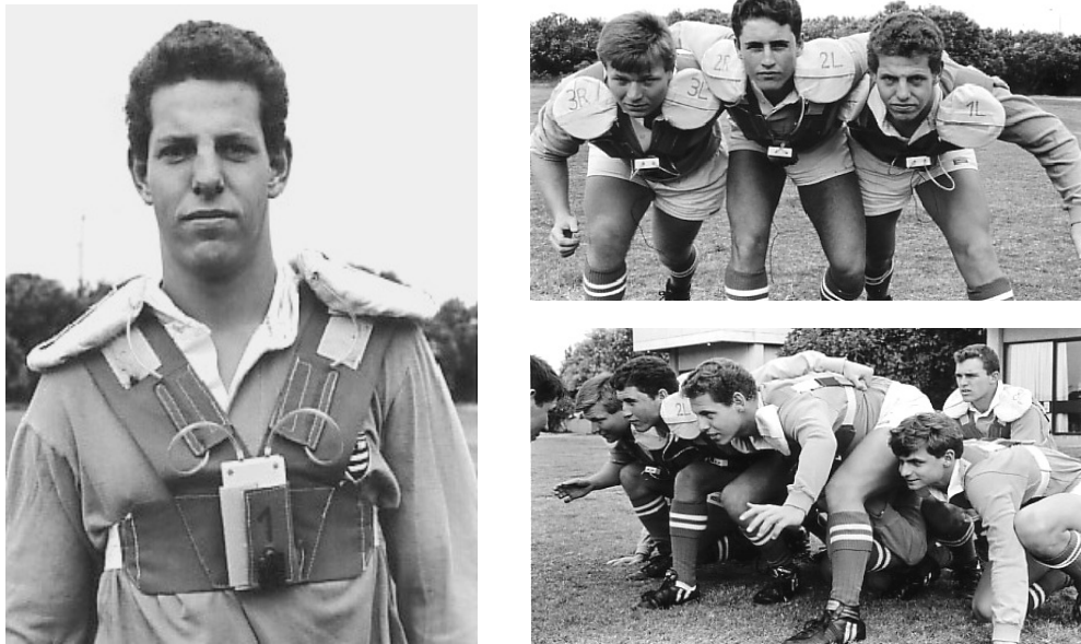
FIGURE 1. THE LIGHTWEIGHT HARNESS FITTED AROUND THE PLAYER'S SHOULDERS AND CHEST WITH ACCOMPANYING PRESSURE PADS AND TRANSMITTER UNIT
