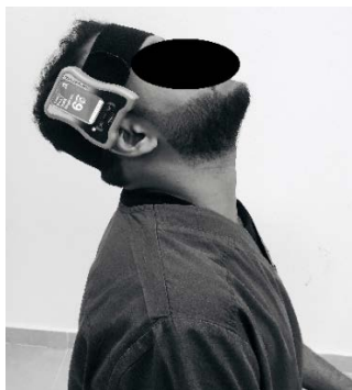
Figure 2. DIGITAL INCLINOMETER MEASURING CERVICAL EXTENSION
