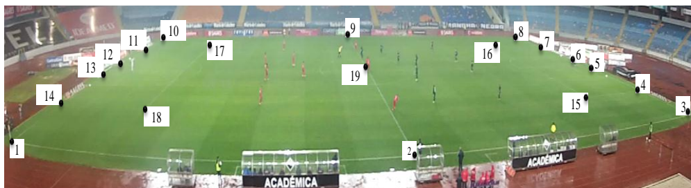
FIGURE 1: INITIAL CALIBRATION TO EXTRACT THE DIRECT LINEAR TRANSFORMATION
