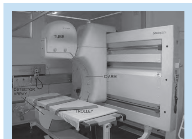
Fig.1. The Statscan machine and its main components.
