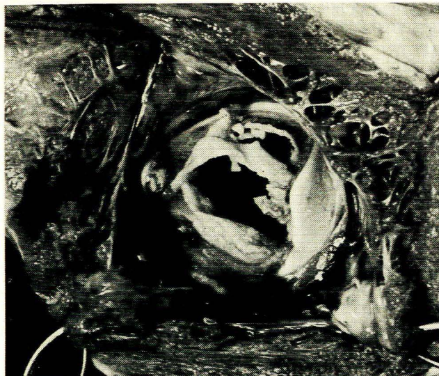
Fig. 3. Teflon prosthesis showing disintegration of a leaflet after 6 months of intracardiac function.
