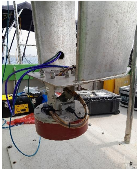
Figure 3: The multibeam Transducer mounted on its Frame
