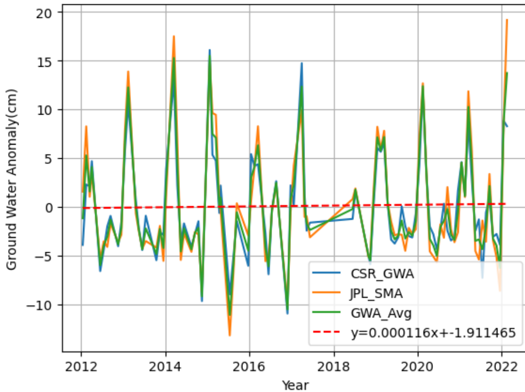
Figure 11: GWA time series with a trend line (red dotted line) representing an upward trend of +0.001mm/year. Average GWA (in green) has been determined from CSR GWA (in blue) and JPL GWA (in orange).
