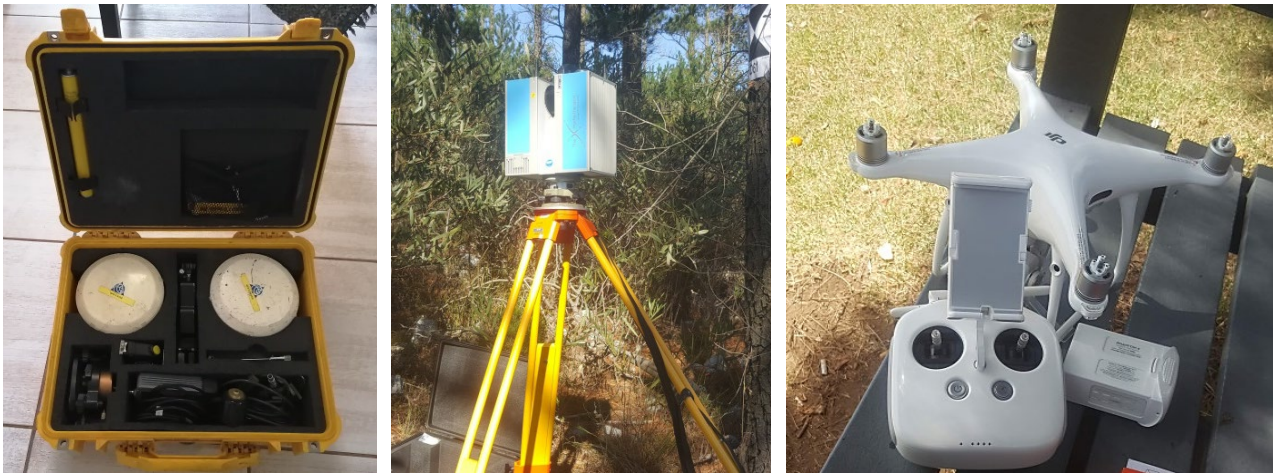
Figure 2. (a) Trimble R4 dGNSS, (b) Z+F Imager® 5010X laser scanner, (c) DJI Phantom 4 Pro Quadcopter
