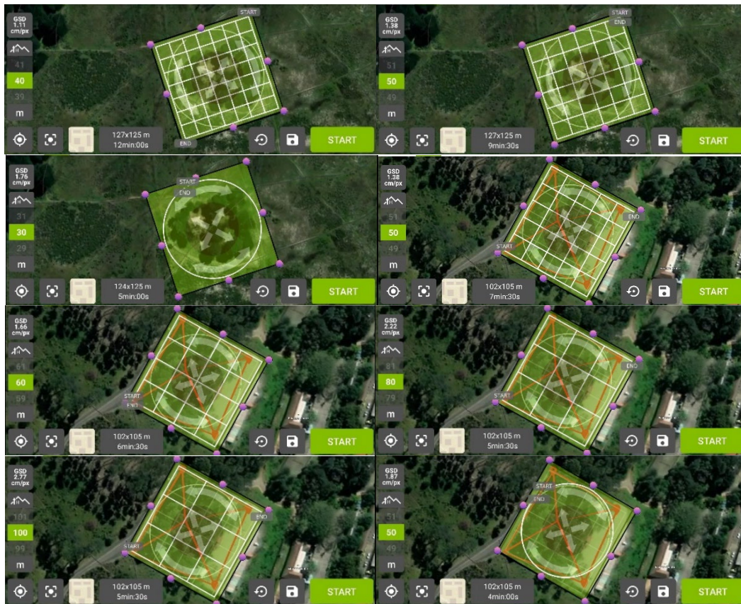
Figure 3. Pix4Dcapture flight plans. (a) – (b) Double Grid Nadir flight for H_{omoFS} , (c) Circular Oblique flight for H_{omoFS} , (d) – (g) Double Grid Nadir flight for H_{eteroFS_1} , and (h) Circular Oblique flight for H_{eteroFS_1}
