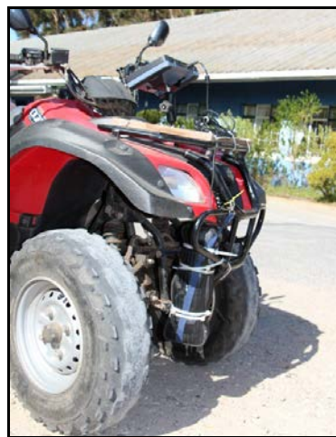
Figure 2. Photograph of the measuring system that was utilised during the in situ measurements. The photograph shows the casing with the detector mounted to the frame and the tablet with an on-board GPS on the carrier.
