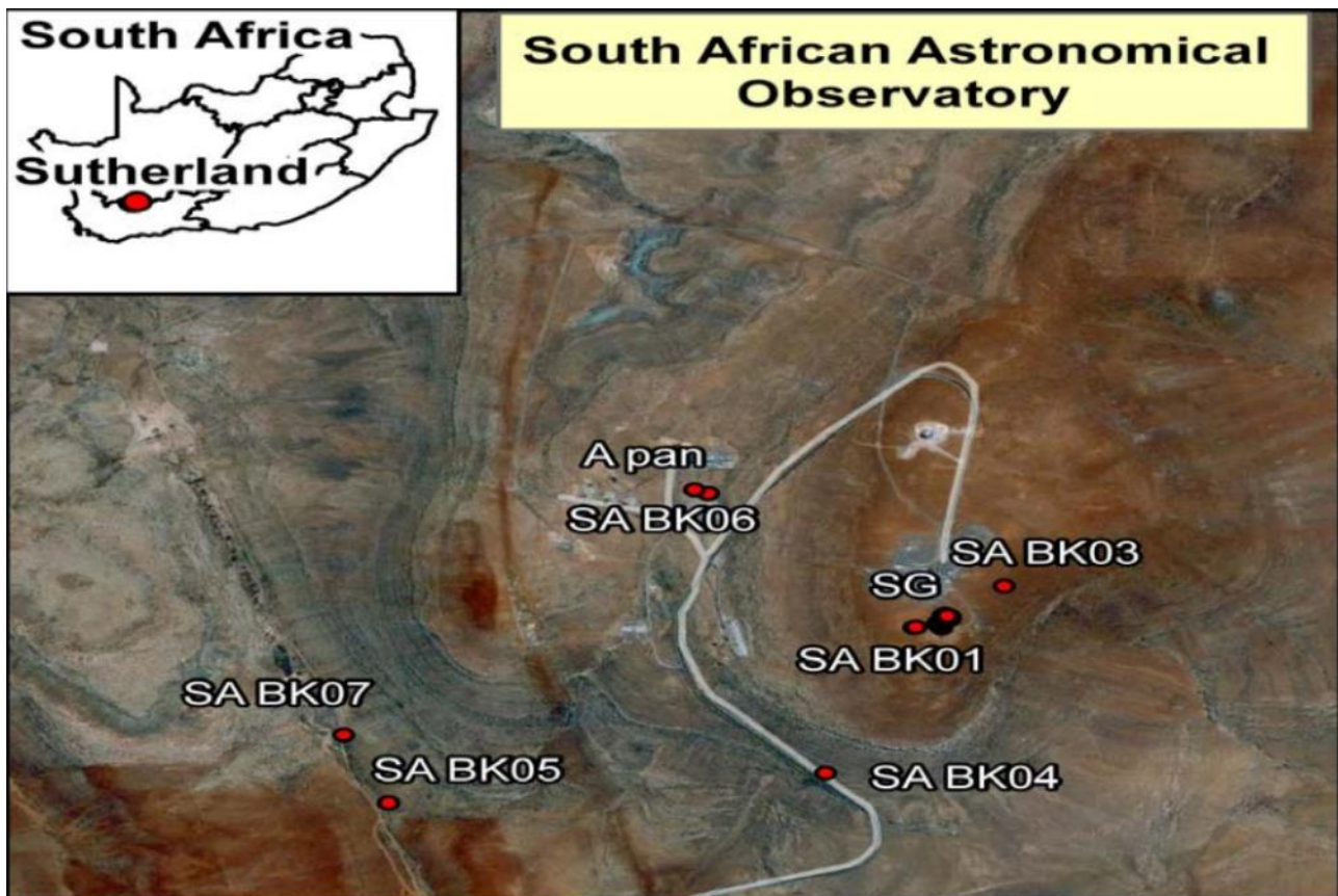
Figure 3. The location of the Sutherland site as well as the layout of the groundwater wells, indicated with SA BK prior to the well number. The site also has an A pan to measure evaporation and the SG located on a hill.
