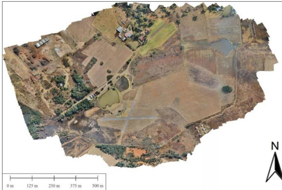
Figure 8. A 10cm ground pixel resolution orthophoto derived from the point cloud for the 100ha study area
