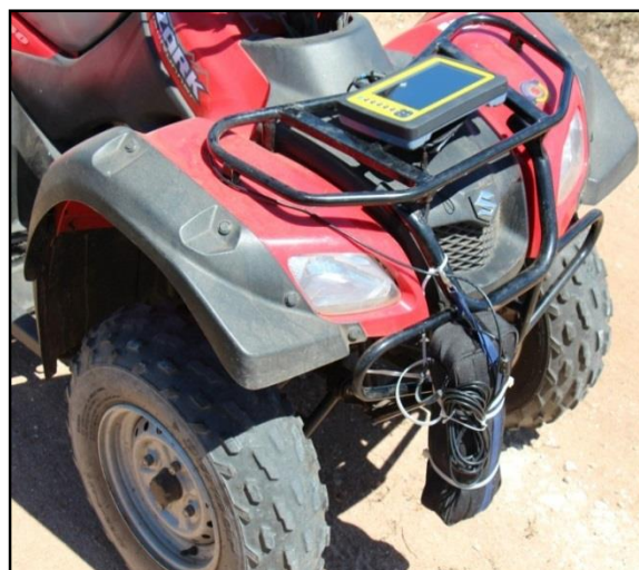
Figure 2: Photographs showing the mounted positions of the GISPI on a quad motorcycle.
