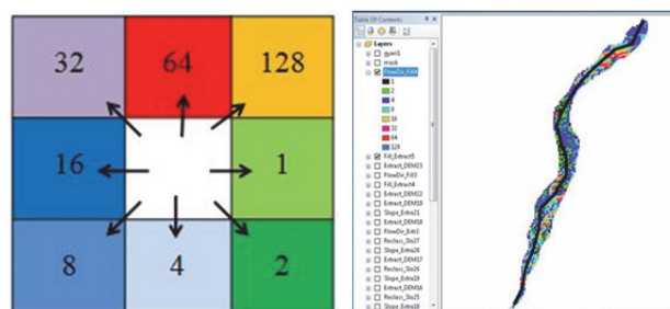
Figure 9. D8 algorithm for calculating the flow direction. Source: ArcGIS software support.
