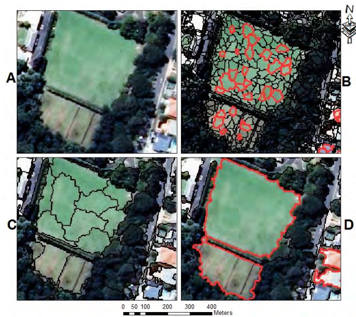
Figure 5: A: Original Kensington scene, 5B: segmentation at scale of 25 showing sport fields partitioned into smaller segments, 5C: over-segmentation at scale of 55 and 5D: good segmentation results at scale of 85.
