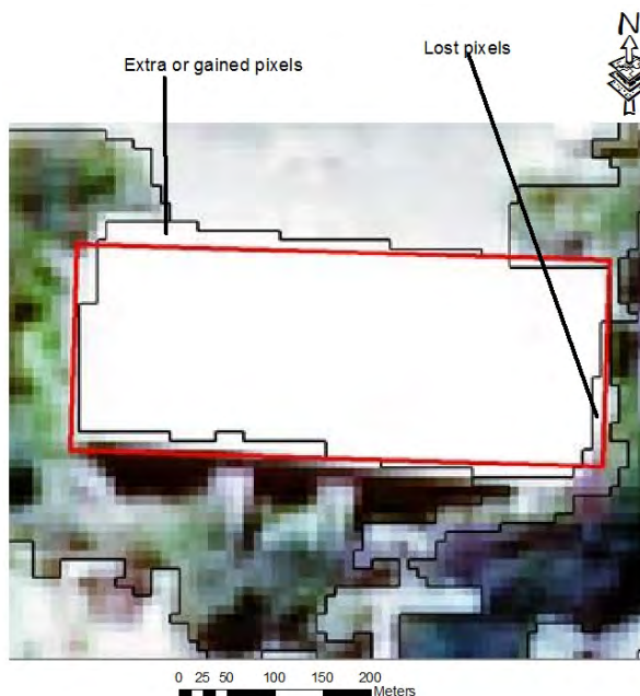
Figure 2: An illustration of a manually digitised reference object overlaid with the segmented object. Gained or extra pixels and lost pixels mostly originate from spectral similarities with neighbouring objects. The areas of lost or gained pixels are characteristics of under segmentation and the percentage area of the biggest segmented object defines over segmentation.
