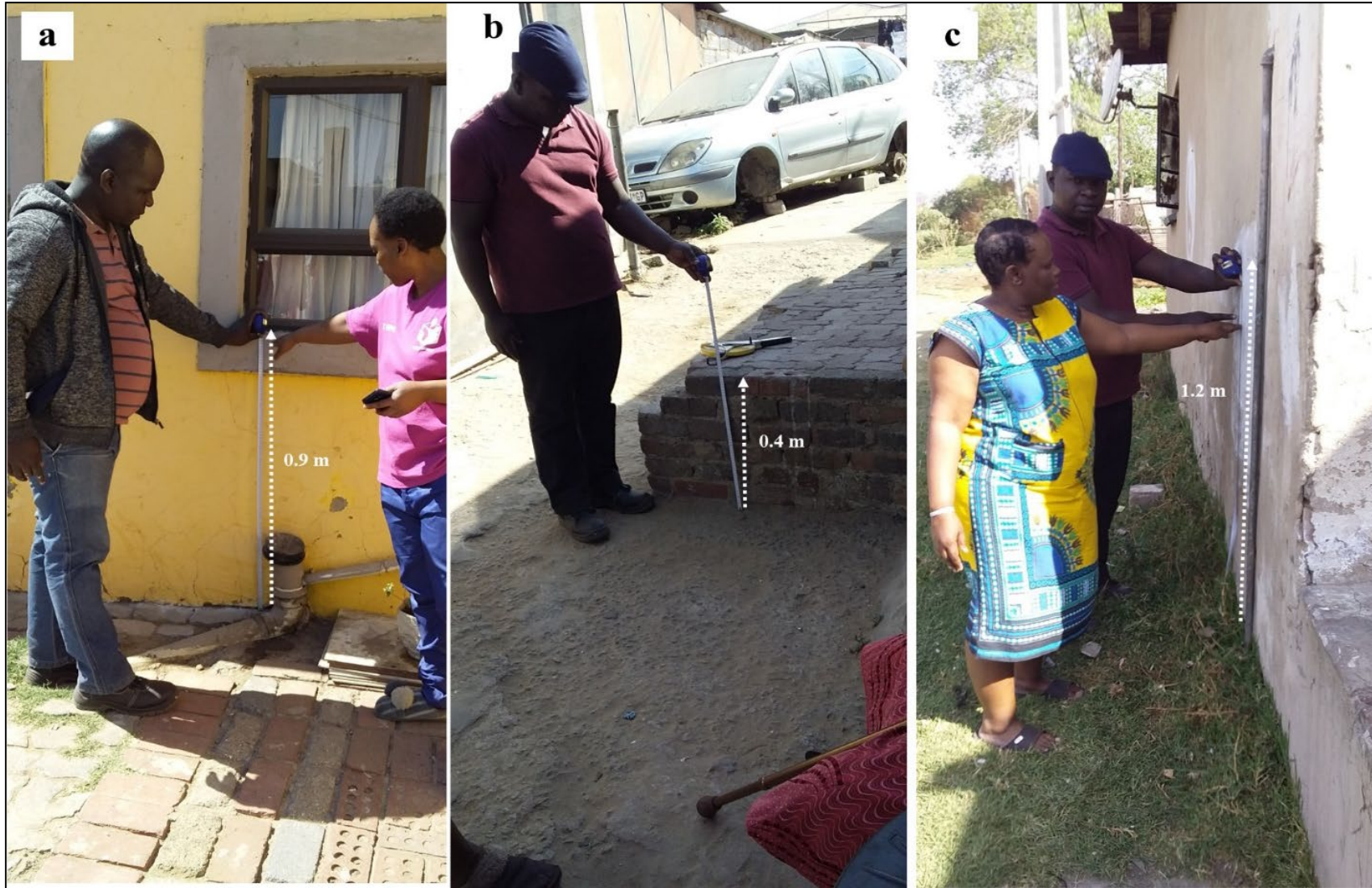
Figure 11: Historic flood water level above ground in various locations along the Jukskei River
