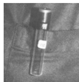
Figure 6 Palmes tube diffusion sampler. 22
