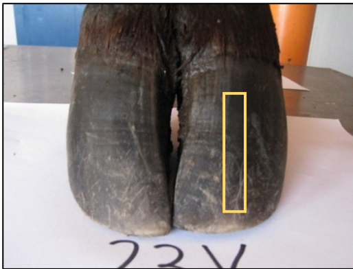
Figure 3 Position of rectangular claw sample on dorsal claw wall for tensile strength testing
