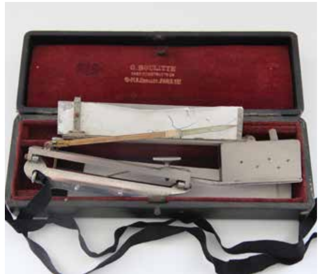
Figure 21a. Marey's sphygmograph for graphically recording the pulse wave c 1860
