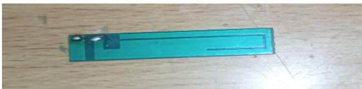
Figure 8: SIM800 GSM MODEM Antenna (Existing antenna).
