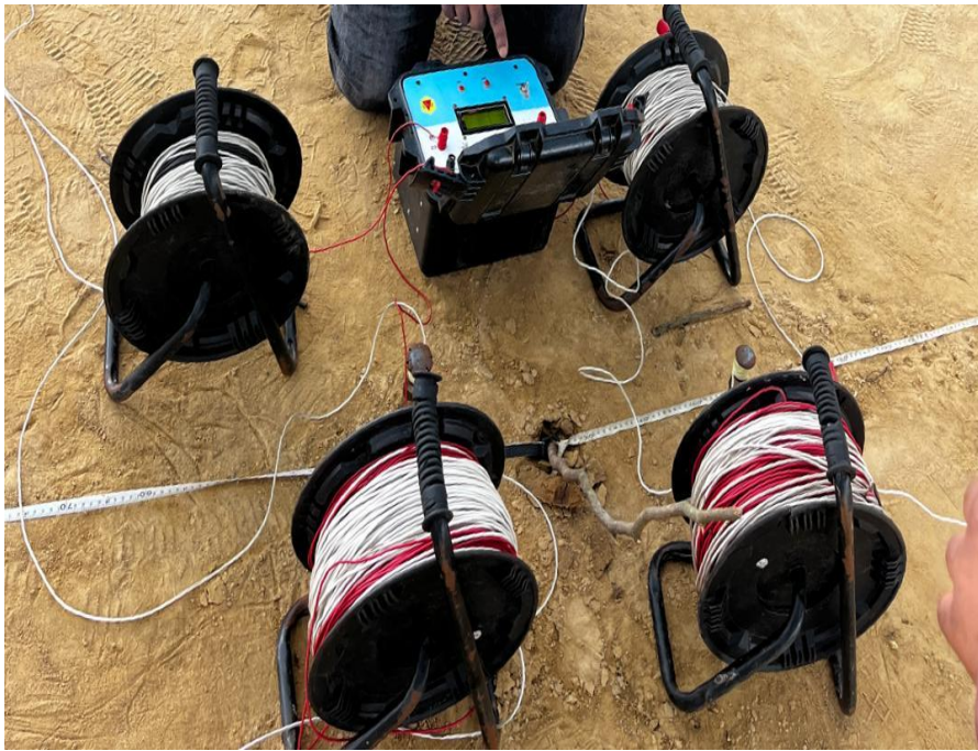
Figure 1: Geophysical Survey Equipment (Terrameter) showing the setup.
