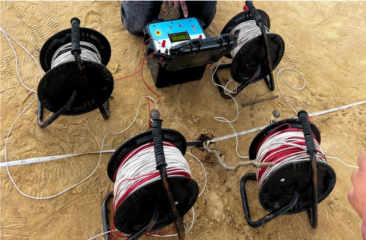
Plate 1: Geophysical Survey Equipment (Terrameter).
